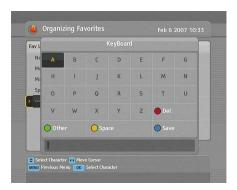
You can move the highlight key horizontally with the ◀ and ▶ buttons and vertically with the ▲ and ▼ buttons. Pressing the OK button on a key enters its letter in the input line. To type a space, select the Space key. To type lower case letters or numerals, select the Other key.
